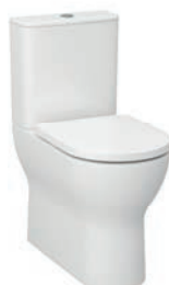
Rimless, comfort height, closed back close coupled pan and cistern (pan height 450mm)
