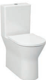
Rimless, comfort height, closed back close coupled pan (pan height 450mm) D 665 x W 360 x H 855mm
